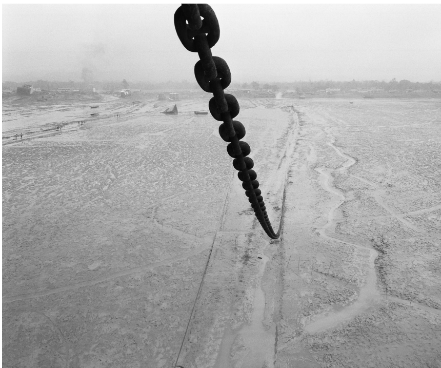
Fig. 20. Anchor chain paid out
