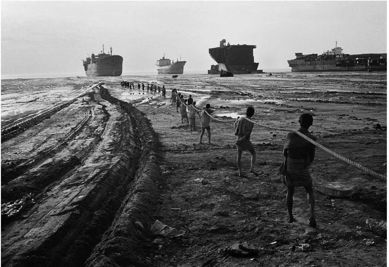
Fig. 16. 'Wire carriers' move cable to the ship to retrieve a felled chunk
