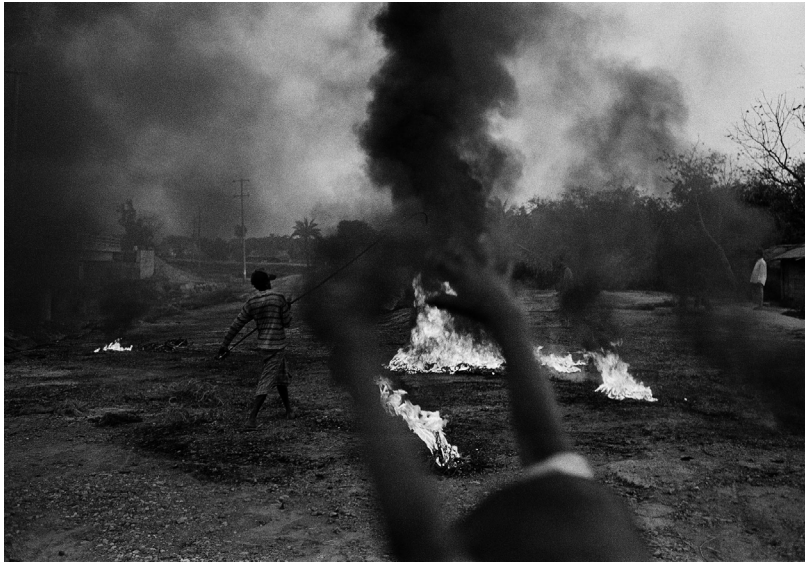
Fig. 29. Burning rubber casting off copper wire
