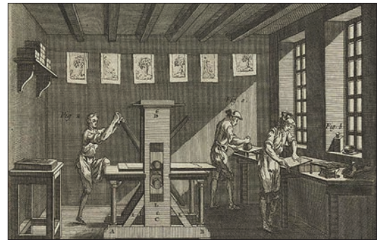
Figure 4: Denis Diderot and Jean Le Rond d’Alembert, Encyclopédie . Vol. 7, plate XIV (showing copper plate rolling press workshop, with copper plate being inked, wiped, and printed).
