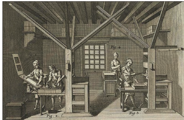
Figure 2: Denis Diderot and Jean Le Rond d'Alembert, Encyclopédie, ou Dictionnaire raisonné des sciences, des arts et des métiers (Paris, 28 vols., 1758-81). Vol. 7, Plate XIV (showing two letterpresses, left with type being inked, right being printed).
